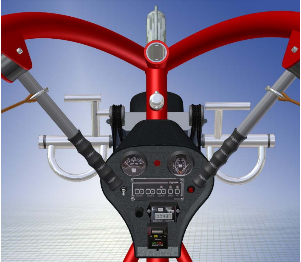
Fig. 2: 3D of XCitor cockpit
