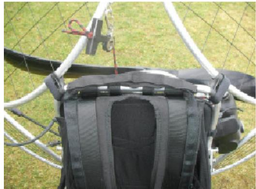
The end of the V-lines are mounted on the carabiners. Check this.
