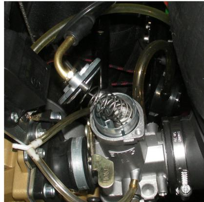
The needle 6L1 is mounted in the second position from top. When replacement is essential to ensure the order.
