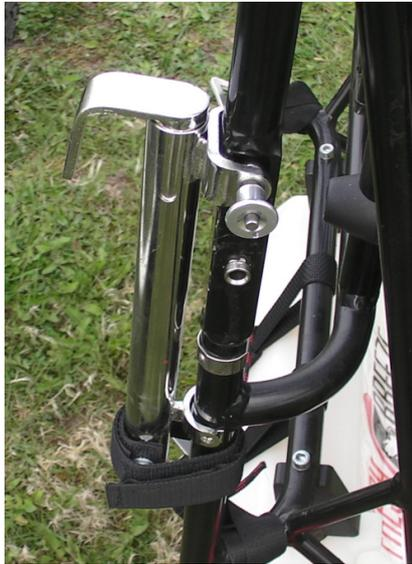
To hang the engine on the trike, put the engine behind the trike and drives it under the hook.
