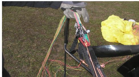
The correct length from the start aid line is essential to check. The red line of the start aid line must sag slightly when the strap is pulled 90° to the push rod. This must be explained/set by an experienced instructor.
