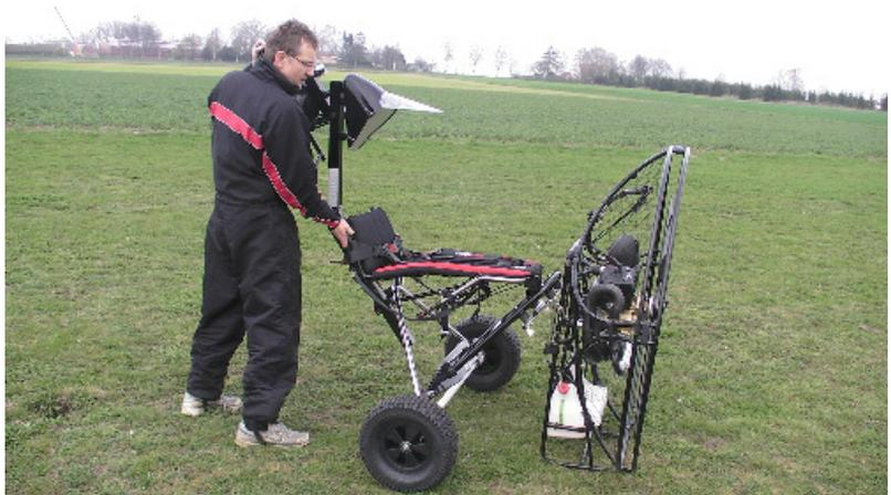
The multi-tubes must fit properly in the white clips. Be aware that the centering pins fit into the holes of the multi-tubes
