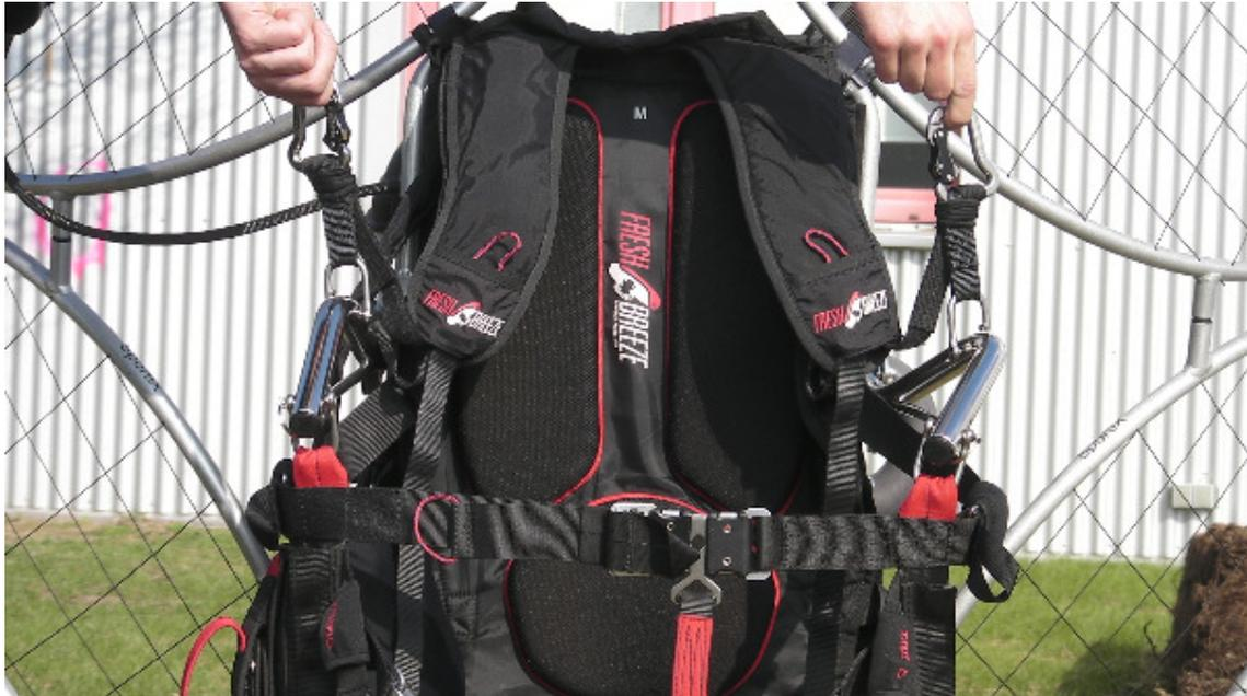
The Super ThoriX has two different pushrods. The left bar is turned outwards. This compensates the negative torque of the engine very effectively. It eliminate the permanent left spin direction in flight when the engine is running under load.
