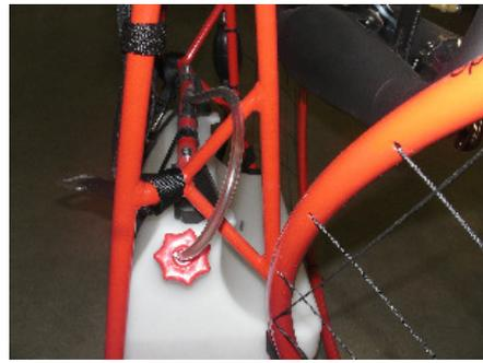
The fuel filter is located below the petrol tank and must be checked before each flight
