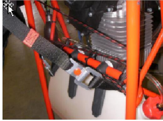
The built in rescue system is integrated into the side of the harness and offers usability and comfort. It is however very important that the reserve bridle runs outside of the pushrods. (See picture). Each time the pushrods are fitted to the frame this needs to be checked.
