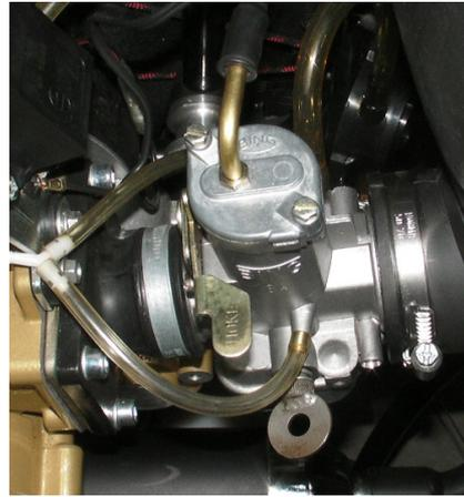
The slider can easily drawn as a whole out of the carburetor. The needle is placed at the lowest position in the slider.
