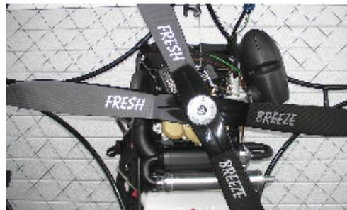
Tighten the 2 blade prop screws M8 x 35 with 10 Nm.
