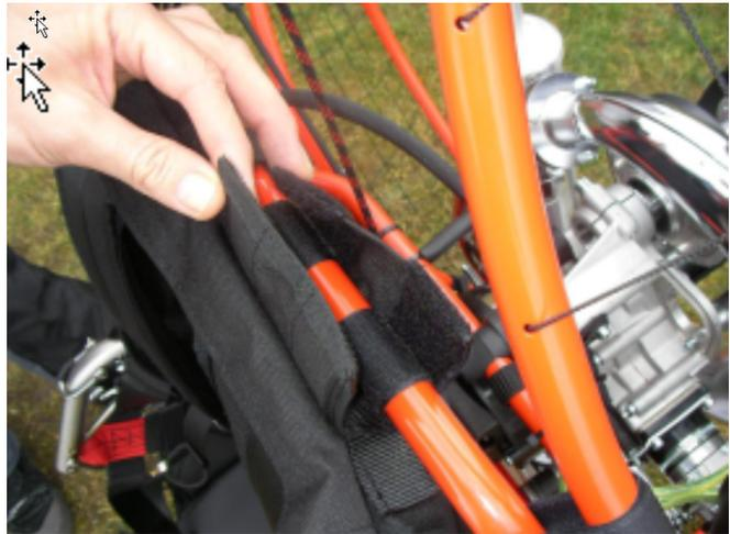
The pushrods are mounted via the quickpins. It is easier if you always leave the quickpins in the pusrods.
