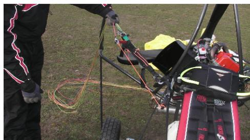
All lines from the glider should be placed in the holder before take off.
