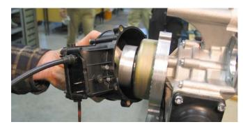
Once the central screw has been removed, the rotor can then be pulled off via a puller. Because the rotor has to be in a specific position to the crankshaft, the rotor with a suspension-disc on the crankshaft is preordained.
