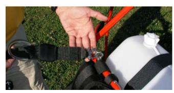
The rear pilotsuspension is adjsutable. For basic position pull the loop until the carabiner. Heavy pilots should open and light weight pilots should close the belt.
