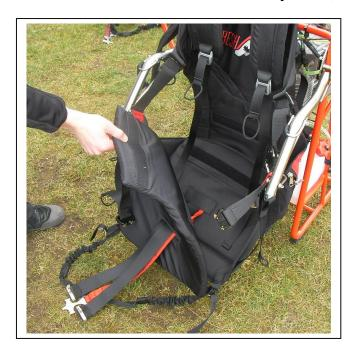
The cage has to be secured on the right side (in flight position) with the help of the extra rubber strap. If your engine is equipped with
