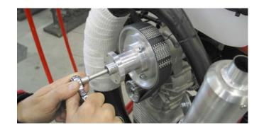
To check the tension turn the belt with your fingers. You should not be able to turn more than 40 degrees.
