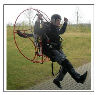
After the start it is recommended to use the supine, to slip into the harness very easy and to take end flight position.
