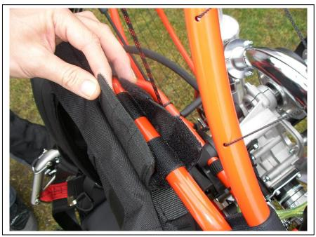
The flexible push bars are fixed with quickpins at the frame. At first you attached the lower quickpin and then the upper one.
