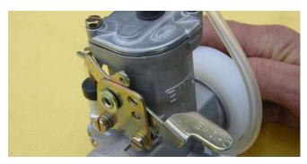
The big screw regulate the idlerunning. Turning right-high rpm. Turning left lower rpm. The idlespeed should round about 240 1/min. The smaller screw is responsible for fuelmixture in idle. Turning right-rich. Turning left-lean
