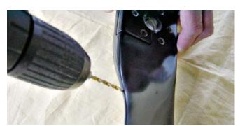
Then fill only as much resign into this hole until the propeller does not want to turn to one side only.
