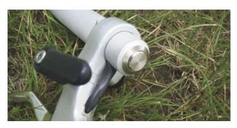
The thottle has also a travelling locking. After reaching the desired hight of flight, the throttle can be fixed via the clasp-lever. Since long holt of the throttle is hard in hand, the throttle can be placed in position onto the legs. The hand are now free for other things.
