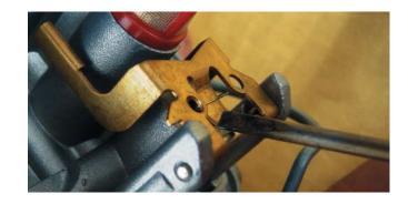
If you hold the carb up side down, the swimmerforc is not parallel to the carburettorcase. If the carb overfloat while using the motor the forc should look a little bit more upward.
