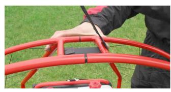
The lowest velcro is sliped through the rails.
