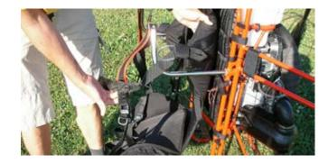
The rear pilotsuspension must fixed in the metal-eyelet.
