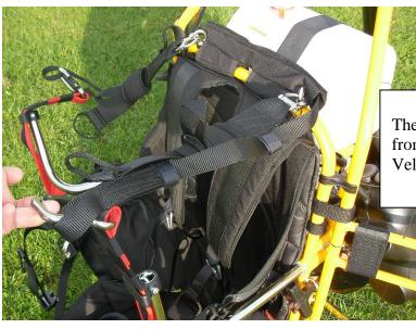
The V cord is led to the carabines from behind and fixed with the Velcro loops.
