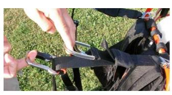
Here you must fix the carringsstraps from harness to the frame.
