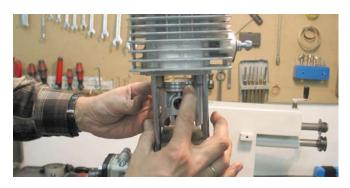
To tighten the headscrews with 14 Nm.
