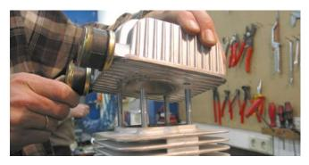
After removing the cylinder you can see the piston. Before you pull out the gudgeon pin remove the safety rings on both sides. Than press out the gudgeon pin.
