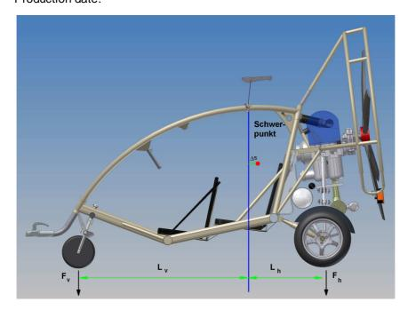
$$\Delta s = \frac{F_{v} + F_{hl} + F_{hr}}{L_{h} * (F_{hl} + F_{hr}) - L_{v}F_{v}}$$
