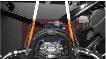
An additional pipe is designed to protect the cage lines at start and landing. After installation of the cage they must hanging in the hub of the rear wheels.
